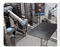
Tray Handling: The stacking of trays on the end of a line or the feeding of trays into a washer is a monotonous and repeatable process that can be easily automated. A robot can be programmed to pick from racks or stack into racks, freeing up your team to engage in greater value-added activities.
