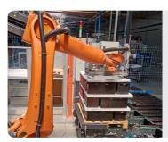
Palletising: Loading products onto pallets from the end of a production line is ideal for robots. This is probably the most common use for robots in the food industry right now and one of the easiest to implement. A perfect example of a repeatable and predictable job for a robot to do 24/7.
